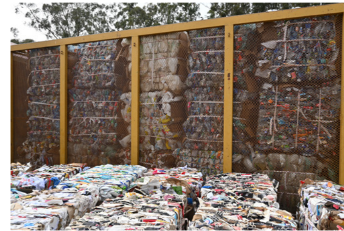
Recyclable materials being baled to increase storage capacity
